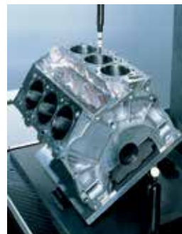
Measurement example of cylinder block and crankshaft.
