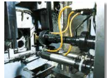
Internal diameter measuring system for lathe post-process
